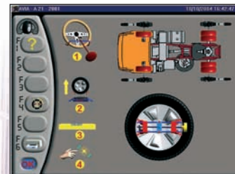
Rolling run-out alignment
